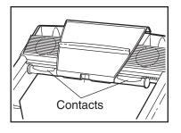
lower left corner of the display will appear, one or two dashes will appear, and then your heart rate will be shown. For the most accurate heart rate reading, continue to hold the contacts for about 15 seconds.
